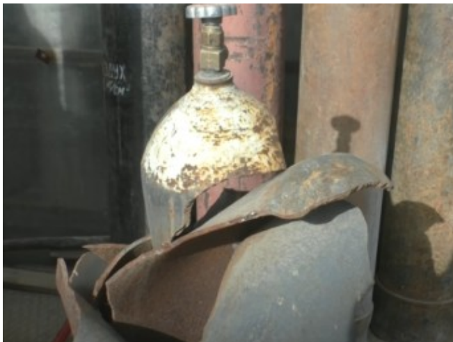
Cylinder rupture after explosion
