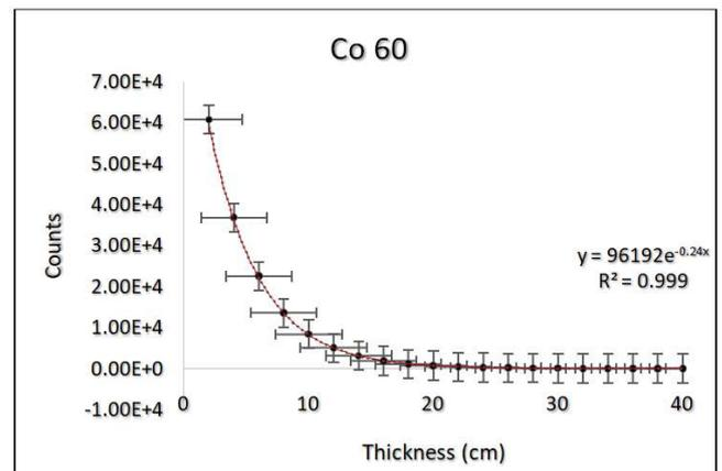
Figure 7. Photon count graphs for Co 60 isotope by target material thickness
