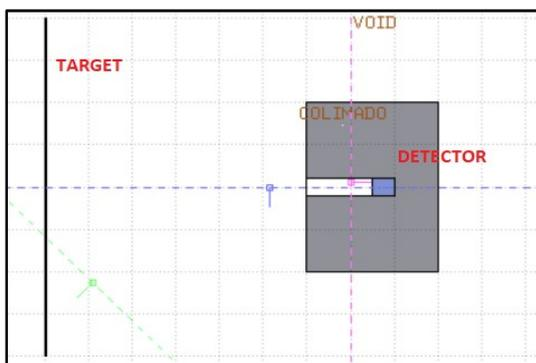
**Figure 1. FLUKA Monte Carlo simulation setup used for mass attenuation coefficients calculations of bismuth oxide-doped glass.**
