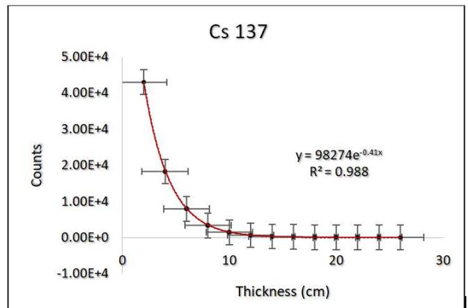
Figure 6. Photon count graph for Cs 137 isotope by target material thickness
