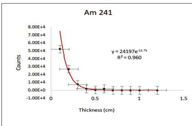
Figure 4. Photon count for Am 241 isotope by target material thickness
