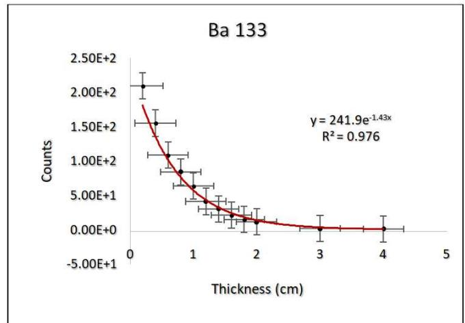
Figure 5. Photon count for Ba 133 isotope by target material thickness
