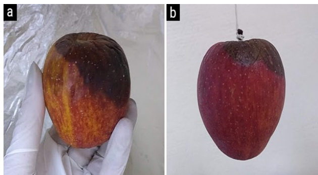
Figure 6. Visual comparison over 12 weeks of Gala apples: (a) without application of coating solution and (b) with application of TPS/1%TiO 2 /0.1%graphene solution
