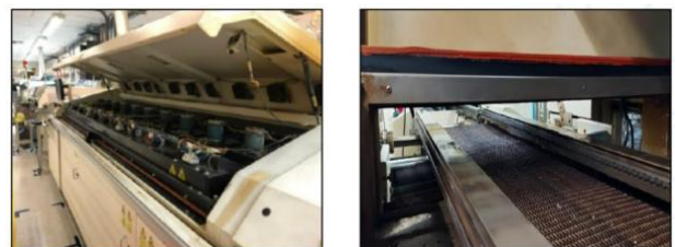
Figure 16. Cleaning the ventilation cooler of the heating zones
