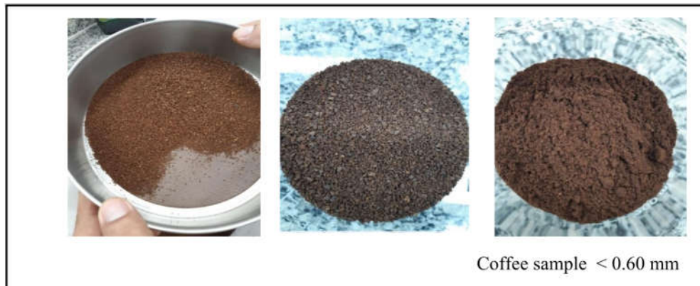
Figure 2. Granulometric standardization of all samples with sieve 28 mesh, (0,6 mm) size
