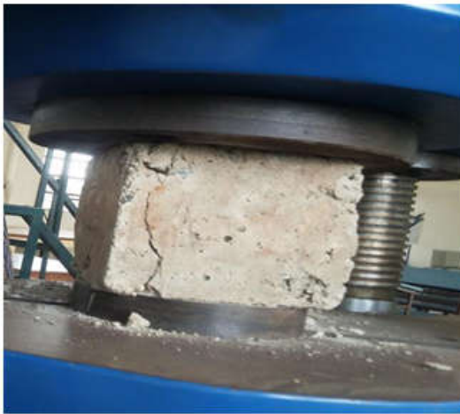
Fig. 4 Compressive Strength Test on Cubes using Universal Testing Machine
