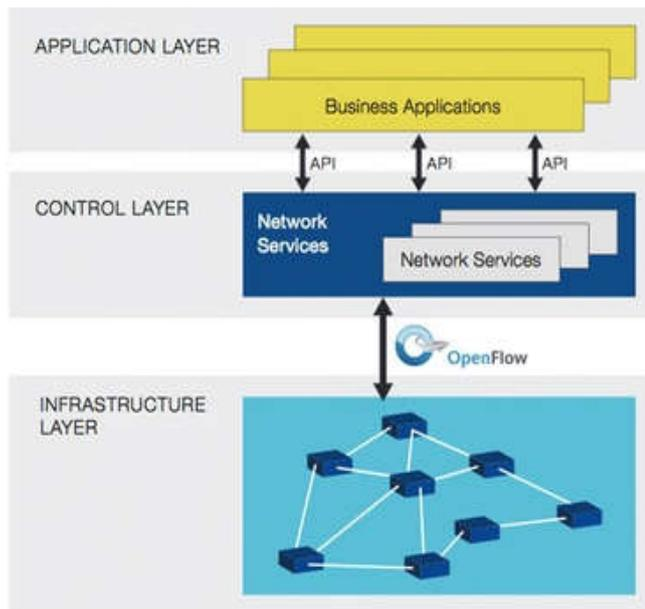
Fig. 1. Software Defined Networking (SDN) Framework
