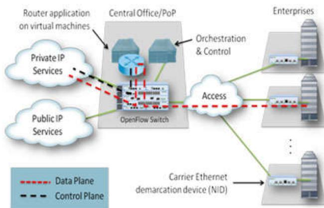
Fig. 2. Sample Network Functions Virtualization NFV deployment
