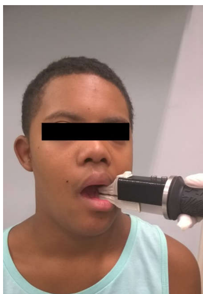
Figure 2. Dynamometer positioned in the region of the first molars on the left side
