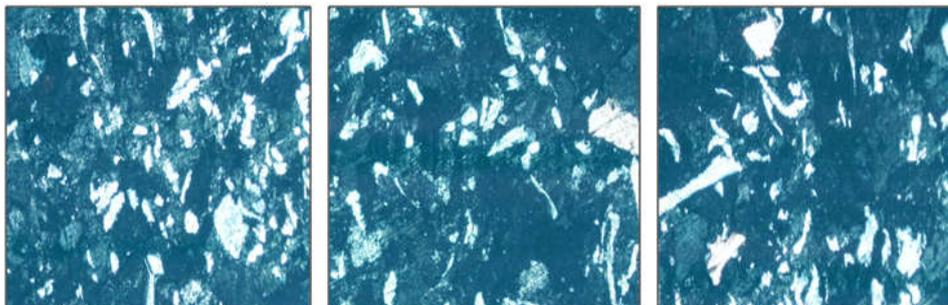
**Fig. 5. Commercial automotive brake pad specimen surface microstructure**
