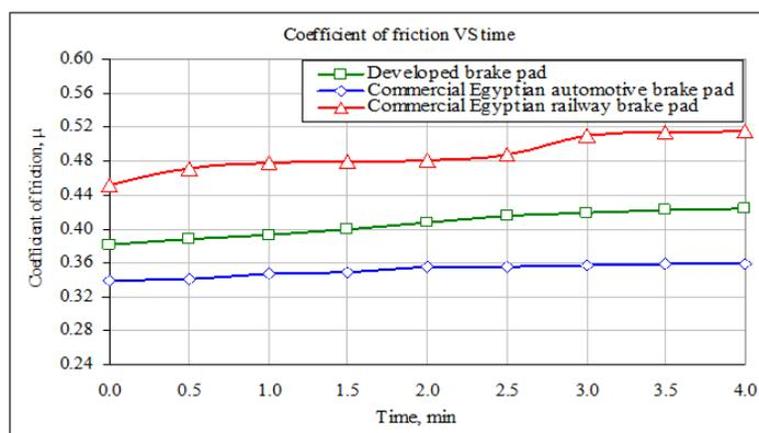
**Fig. 2. Comparison of coefficient of friction of the specified brake pads**
