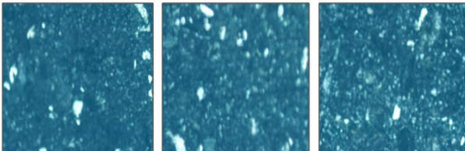
**Fig. 4. Commercial railway brake pad specimen surface microstructure**
