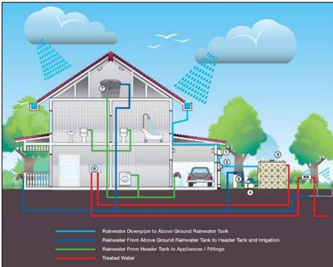
Fig. 3. Above ground rainwater harvesting system: 1. Lift filter, 2. Downpipe first flush diverter, 3. Above ground rainwater tank, 4. Automatic booster pump, 5. Sand bedding filter, 6. Rain backup in a box, 7. Header tank. (Aura-Lite, 2015)
