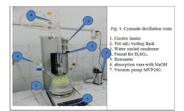
Fig.1. Cyanide distillation apparatus
