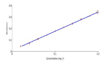
Fig.3.5. Calibration curve of the CN<sup>-</sup> concetrations
