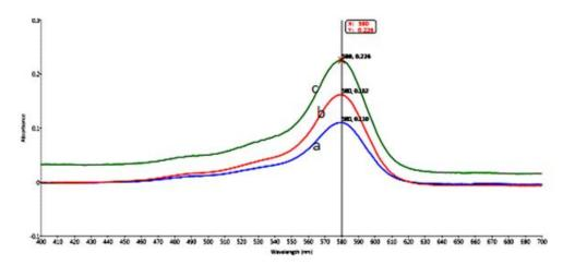
Fig.3.1. UV- pyrazole blue spectrograms with different concentration of CN<sup>-</sup>: a. CN<sup>-</sup> = 0.04 mg/L; b. CN<sup>-</sup> = 0.06 mg/L; c. CN<sup>-</sup> = 0.08 mg/L.
