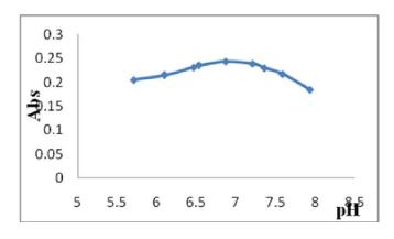
Fig.3.2. Dependence of absorbance on pH in the range from 6.53 to 736
