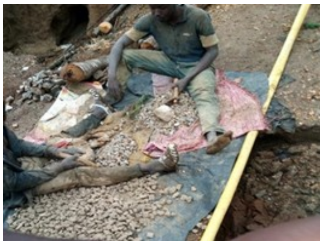
Figure 5. Manual crushing using a hammer
