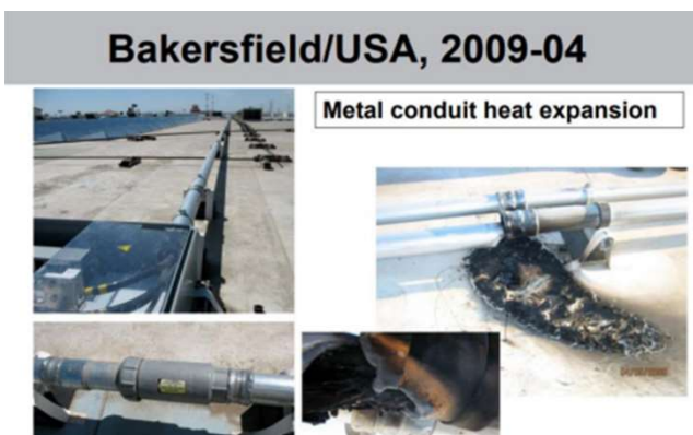
Figure 10. Arc in the metal conduit due to insulation issues with the cables
