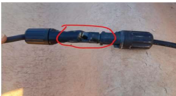
Figure 20. Faulty MC4 Connector in String 5
