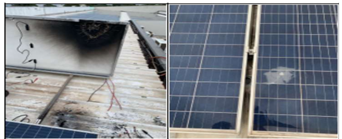
Figure 7. Fire in PV Solar Panels due to an Electrical Arc
