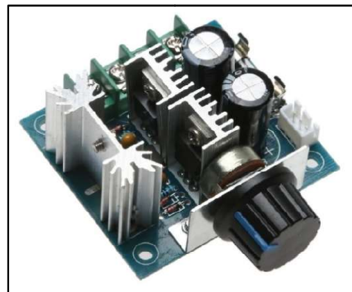
Figure 4. DC Motor Speed Governor PWM Controller DC 12V 24V 30V 40V 13KHZ [8]
