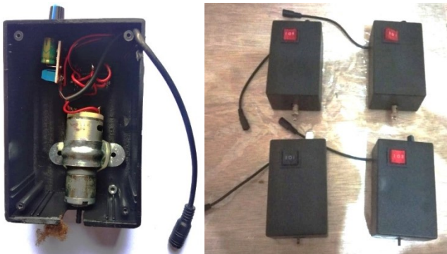
Figure 7. Speed controller and geared DC motor is packed in a fix box
