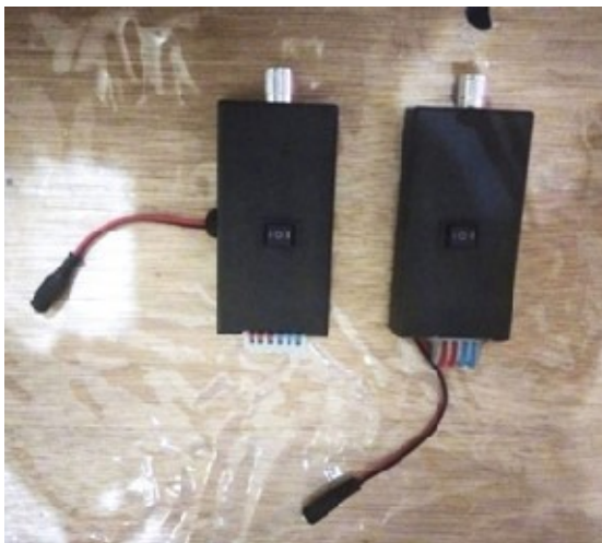
Figure 8. Speed controller and switch reverse rotation is packed in separated box to the geared DC motor to enable it to operate at a distance
