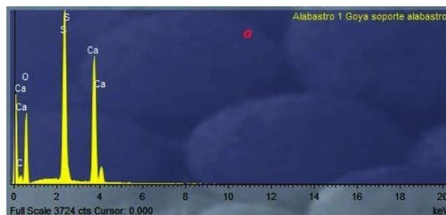
**Figure 3a.** Spectrum obtained via SEM-EDX microanalysis, with the characteristic peaks of gypsum that makes up the alabaster medium.
