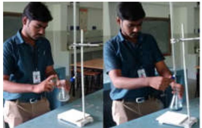
Figure 1. Identification of Calcium Carbonate by Titration Process
