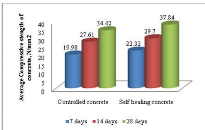
**Figure 3. Comparison of Compressive strength of Controlled and Self healing concrete**
