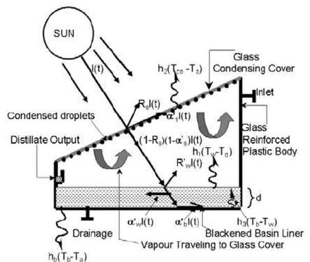
Fig. 1. Cross-sectional view of schematic arrangement and various energy transfers [35]
