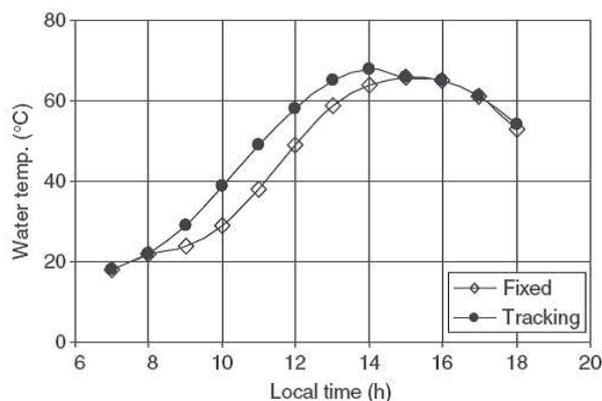
Fig. 3. Temperature variation of the water basin for both fixed still and still with tracking system [108]
