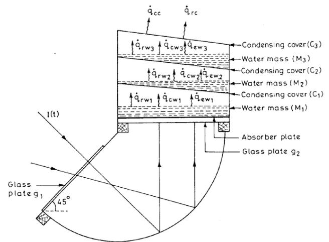
Fig. 2. Schematic diagram of an inverted absorber triple effect solar still [58]
