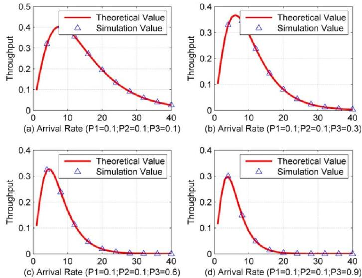
Fig. 6. The throughput of the new protocol with different  $P3$
