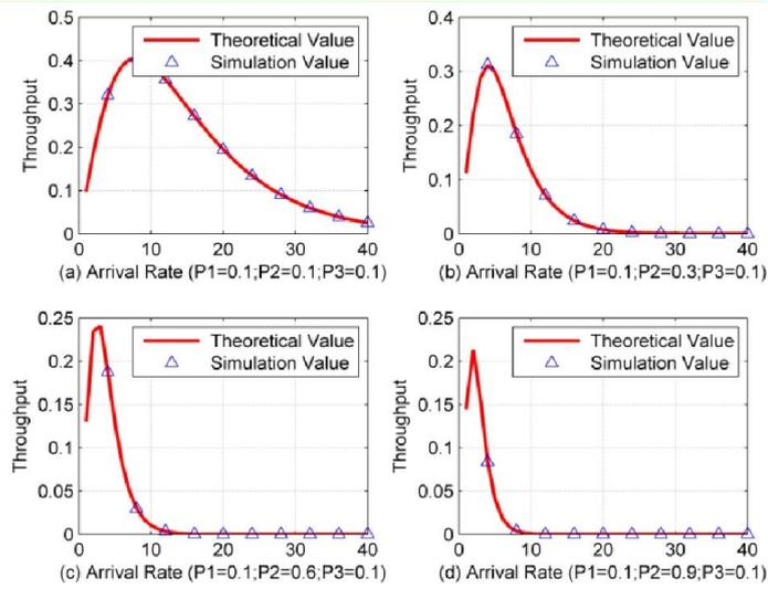
Fig. 5. The throughput of the new protocol with different  $P2$
