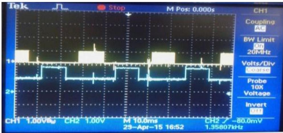
Fig. 10(a). Waveform of PWM at speed 400 rpm
